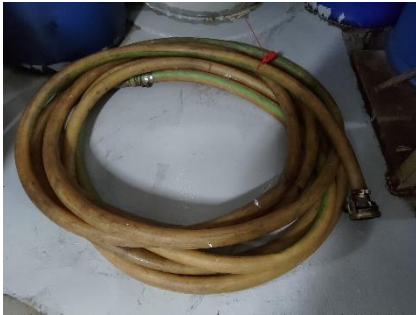
Hose for hold / deck washing tagged
